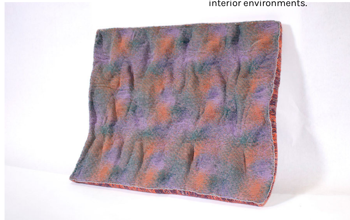
Multi-layer Jacquard-woven fabrics designed as acoustical panels for interior environments.
